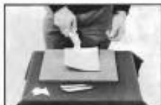
4. Ensure that the work surface is glue free. Then place rubber, playing face down, on the board and apply glue. If the rubber is covered by a protective paper it is wise to leave this in place.
